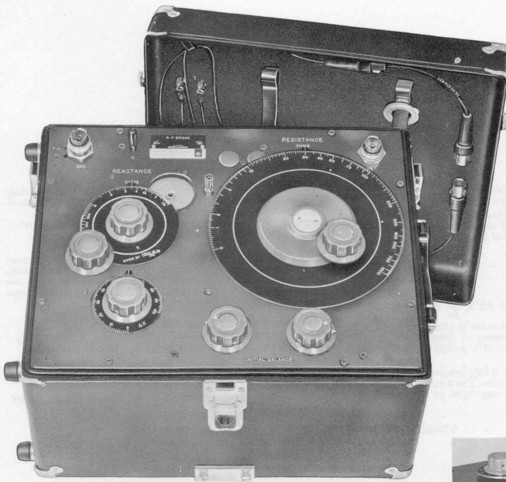
View of the Type 916-AL Radio-Frequency Bridge showing panel controls
